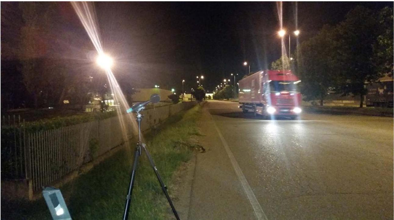
A nighttime photograph of a road scene. A red truck is driving towards the camera on the right side of the road. In the foreground, a microphone is mounted on a tripod on the grassy shoulder. The road is lit by streetlights, and a fence is visible on the left. |    |                        |          |
